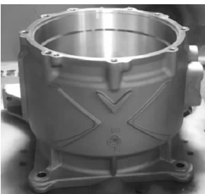
图 12 按照改进后工艺方案制备所得电机壳实物图 Fig.12 Entity of motor shell produced according to the modified production process
