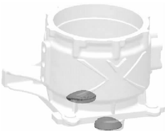
图 11 改进方案的缩孔缩松缺陷模拟结果 Fig.11 Simulation results of shrinkage cavity and porosity under modified design condition
